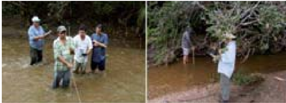
Photo 2.12 – Discharge measurement at key-curve calibration stage.
