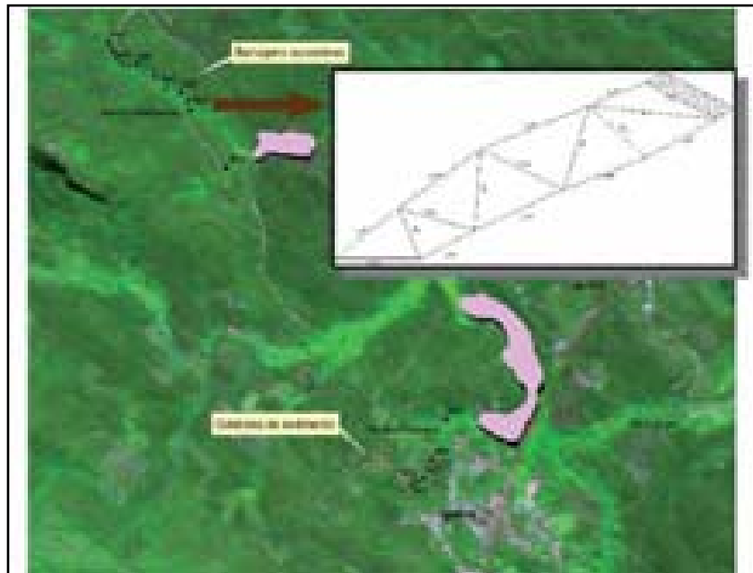
Figure 2.114 – Plan to estimate the surface area of sediment accumulation in B11 dam
