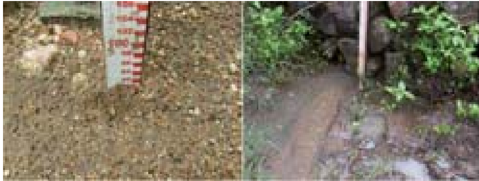
Photo 2.09 – Limnometric rulers installed in successive dams monitored by subproject..
