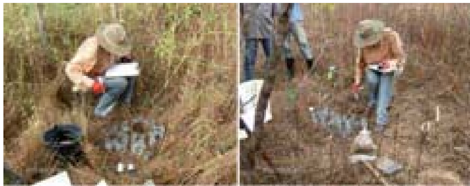
Photo 2.11 – Infiltration essays using “Beerkan” method
