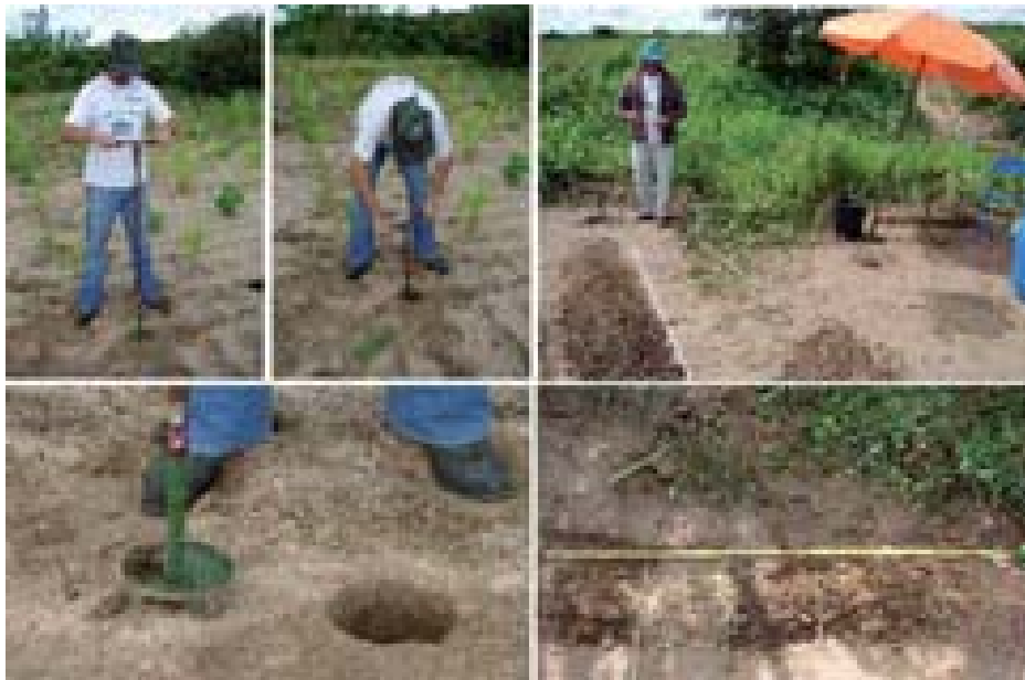
Photo 2.19 – Auger drilling stages during field works.
