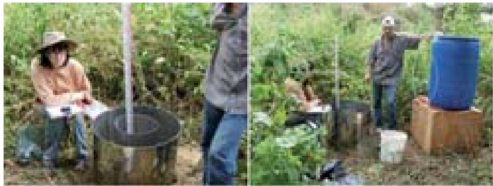
Photo 2.10 – Infiltration essays using concentric rings
