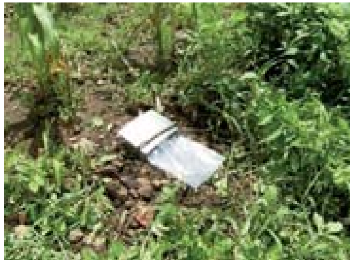
Photo 3.05 – View of a soil and water collector assembly
