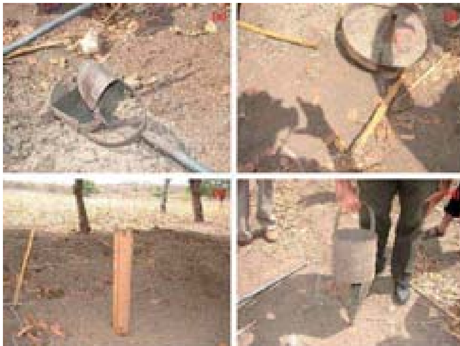
Photo 2.20 – Equipment used for alluvium drilling: (a) stone collector; (b) dry sand glass; (c) buster; and (d) argillaceous material glass.
