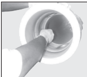
Cleaning inside the vessel
