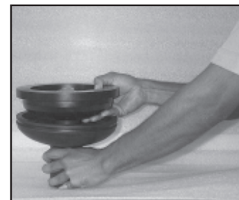
Removing the Elliptical Metal Dish
