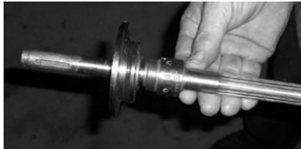
Figure 7-30 – Install seal and seal plate onto shaft
