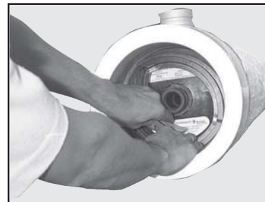
Installing Locking Segment
