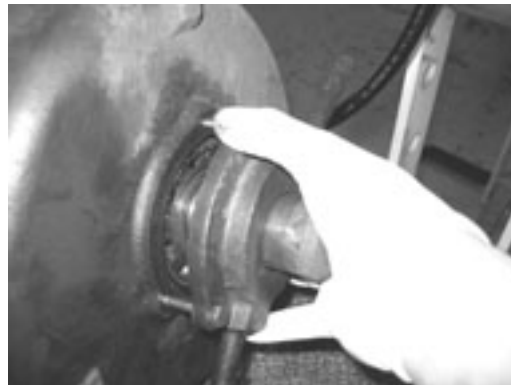
Figure 7-45 – Remove Bearing Lubrication Covers
