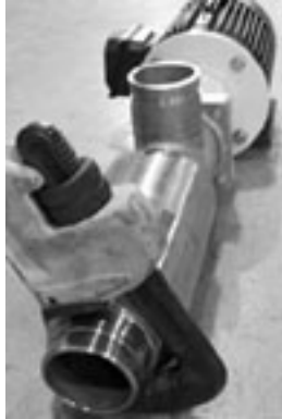
Figure 7-26 – Loosen Outlet Nozzle
