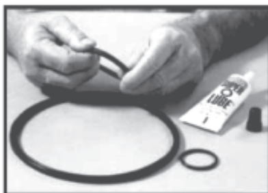
Lubricating Head Seals & O-rings
