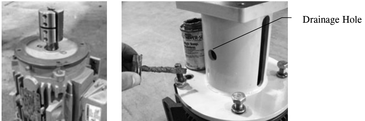
Figure 7-11 – Install Coupling and Bell Housing onto Motor
