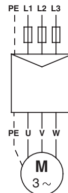
Fig. 14 Grundfos motors, direct-on-line starting
