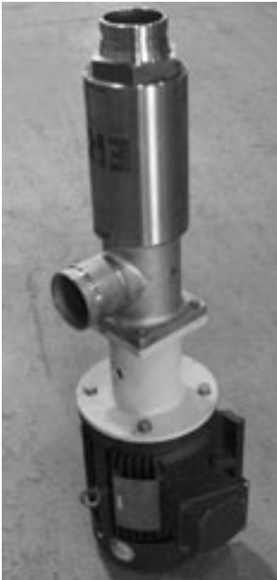
Figure 7-4 - Remove Pump from Bell Housing
