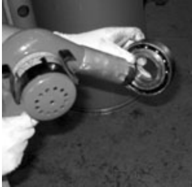
Figure 7-50 – Heat Inner Ring to 180°F (82°C)
