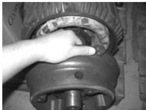
Figure 7-46 – Remove Front Bell
